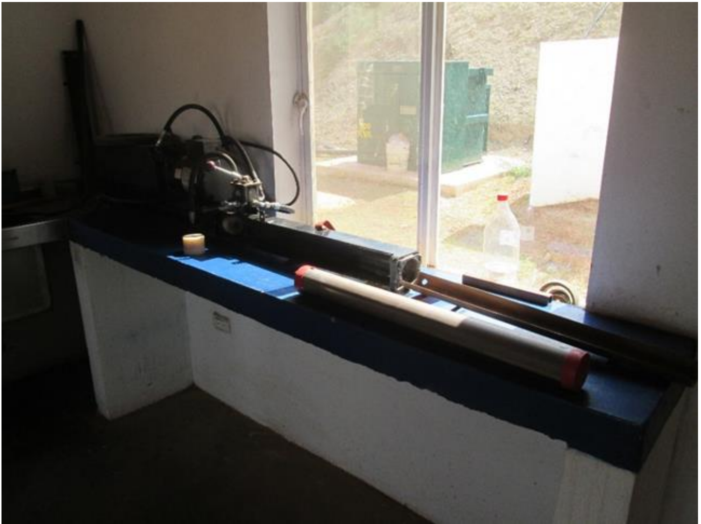
Figure 12-4: Logging and Sampling Facility – pneumatic piston and capped sample tube
