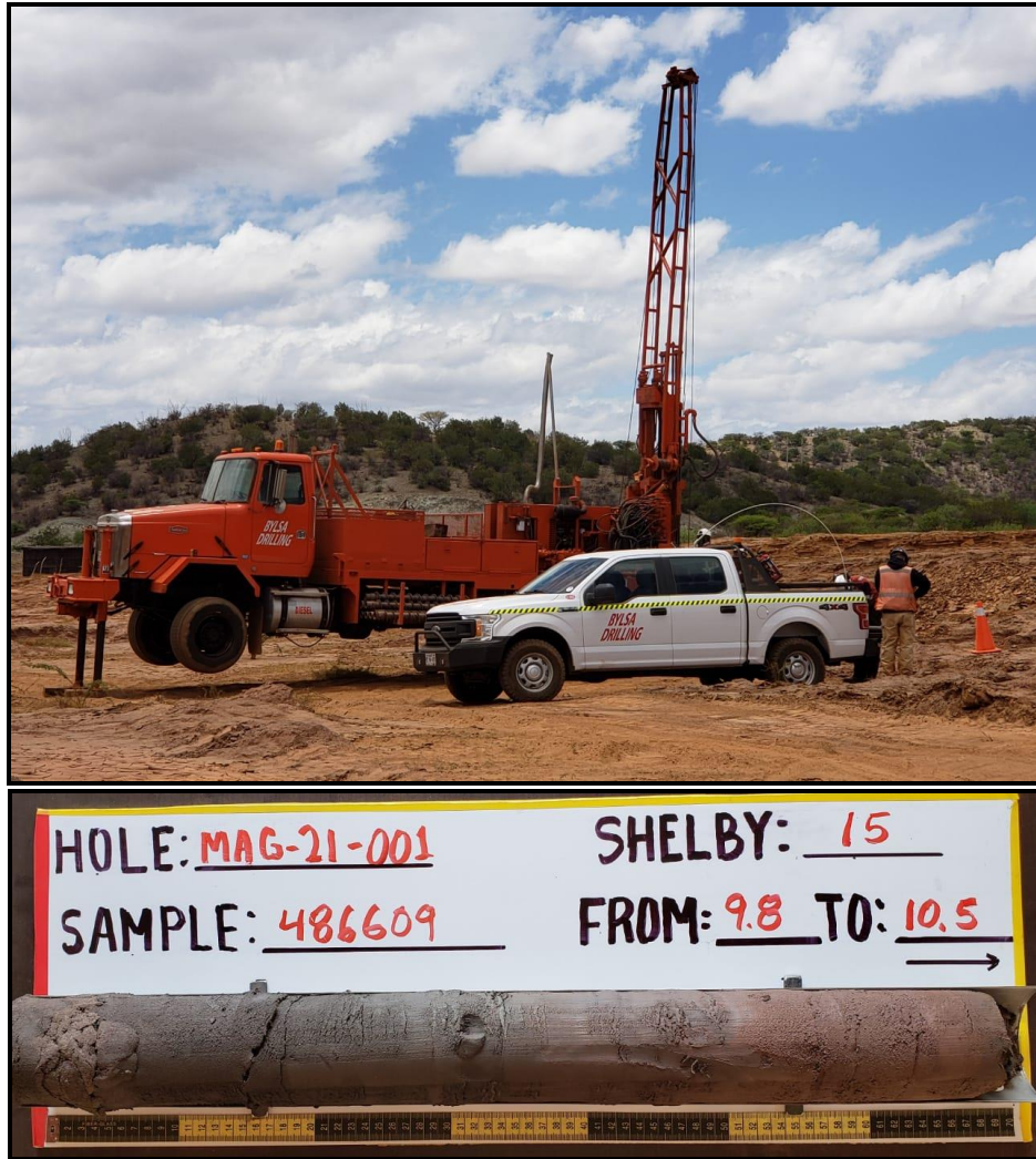
Figure 2 – Auger Rig and Tailings Sample from Magistral
